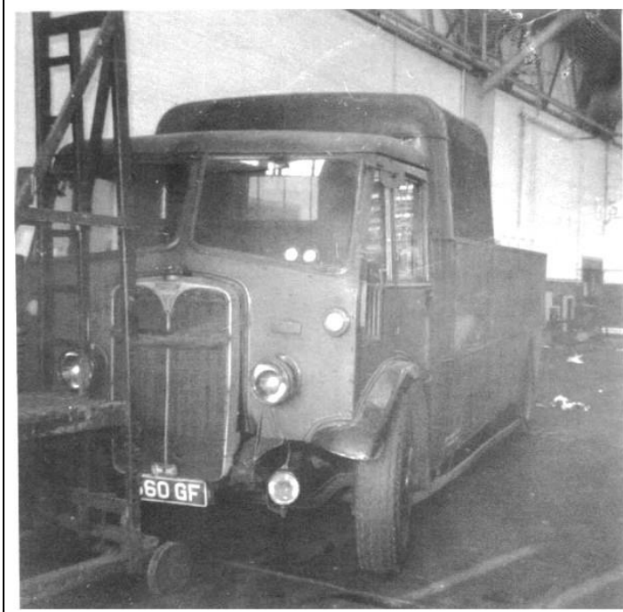
Photo 241, by Clive Greedus , added to LTSV on 15/12/2003. Seen parked out of use inside Upton Park bus garage in March 1964 is AEC Regent towing lorry 811J, converted from bus STL377 in 1950. Note that the rebuild included the provision of a full-width cab. This vehicle was sold three months later in June 1964.
