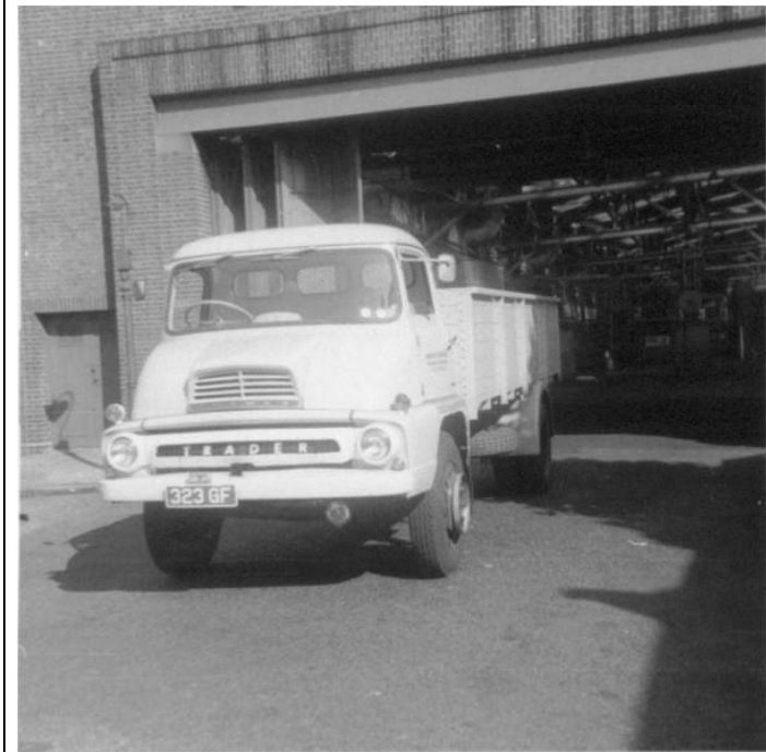
Photo 242, by Clive Greedus , added to LTSV on 15/12/2003. Upton Park bus garage in March 1964 and parked outside is 3 month old Thames Trader towing lorry 1309F. Such vehicles were readily recognisable by having fixed sides rather than dropsides. This vehicle replaced 811J as the resident tow truck.
