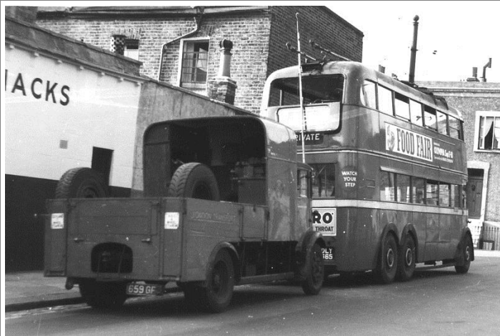
Photo 1941, by Alan B Cross , added to LTSV on 07/06/2007. A rear view of Albion KN127 Trolleybus Rescue Truck 124A shows the covered area complete with workbench, and the spare wheels. As well as the central drop-down flap, the rear also featured two tall, narrow doors (seen here with white plates attached) that opened to form ramps for the unloading of wheels. Although bought in the late 1930s, most of these vehicles survived until the end of the trolleybuses in 1962. Reproduced by kind permission of Alan Cross. Copyright.
