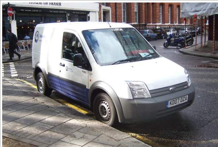
Photo 1974, by Ray Monk , added to LTSV on 01/07/2007. The Ford Transit Connect received a minor facelift during 2007, with a revised front bumper and radiator grille, and the Ford badge moved down from the bonnet. Illustrating these changes is Tube Lines operated 6217F, found at Howick Place (off Victoria Street) on 22nd June 2007.
