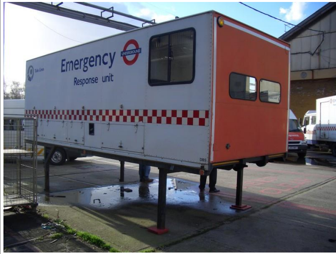
Photo 1872, by Thomas Young , added to LTSV on 22/04/2007. Opposite the main ERU building within Acton Works on 6th March 2007, spare demountable body DB5 was standing on its own legs, these being the ones without shoes on! The orange stripes at the bottom of the front end may be used by drivers when backing chassis underneath at night.
