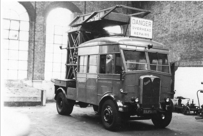
Photo 1939, by Julian Bowden-Green collection , added to LTSV on 07/06/2007. Rarities among the tower wagon fleet were a pair of AEC Monarchs bought in 1938 instead of the more usual Mercury model. At this time, different types from the same manufacturer were sometimes given different fleetnumber suffixes. N was assigned to the AEC Monarch, and carried by just the two tower wagons and a trio of pole carriers. 100N was found resting in Lea Bridge depot.
